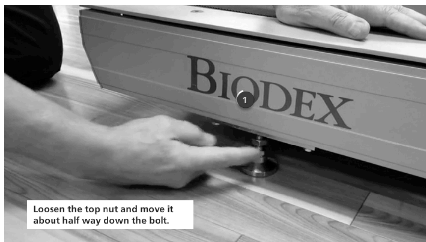
Figure 1.2. Loosen the Top Nut
