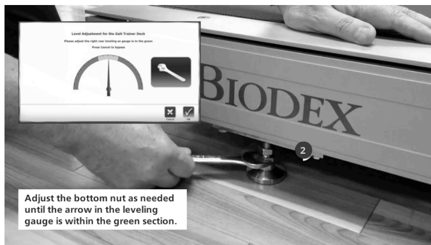
Figure 1.3. Adjust the Bottom Nut
